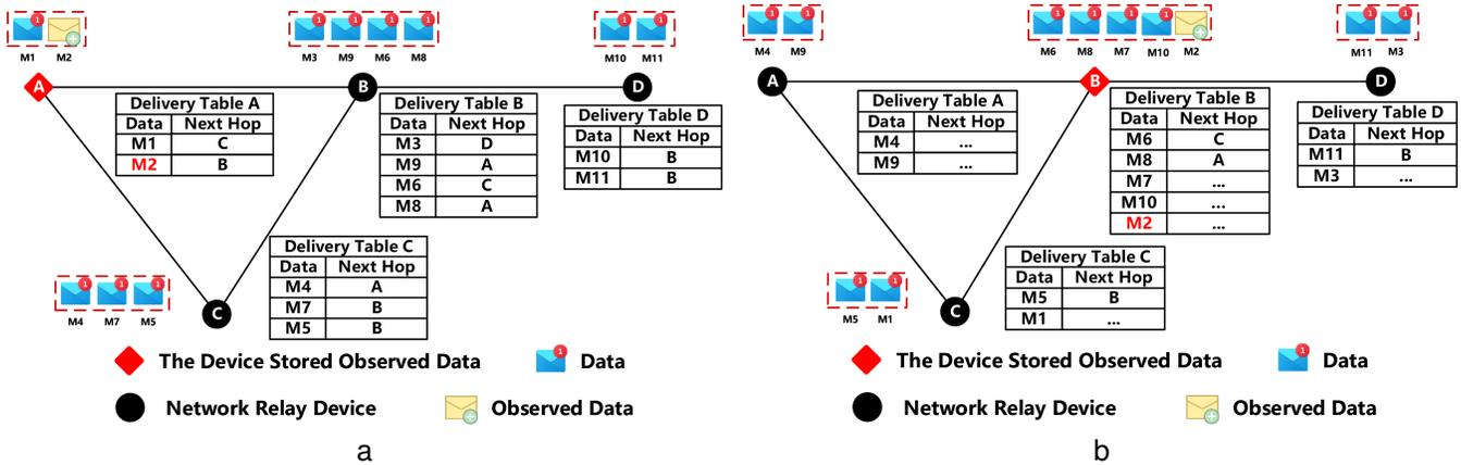
Fig. 3. An example of calculating predicted buffer time  $T_r^{t+1}$  in period  $t$ . (a) The data  $m_2$  is in the origin device  $r_A$ . (b) The data  $m_2$  is in the network relay device  $r_B$ .
