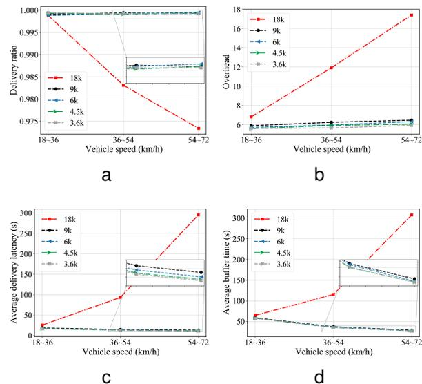
Fig. 9. (a) Delivery ratio versus vehicle speed. (b) Overhead ratio versus vehicle speed. (c) Average delivery latency versus vehicle speed. (d) Average buffer time versus vehicle speed.
