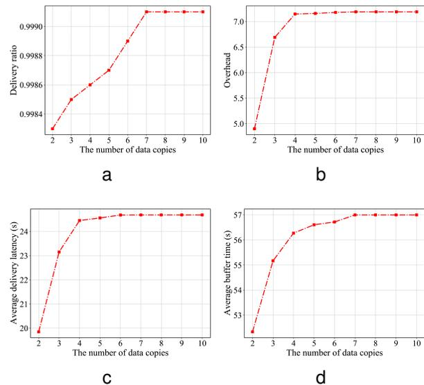
Fig. 8. (a) Delivery ratio versus the number of data copies. (b) Overhead ratio versus the number of data copies. (c) Average delivery latency versus the number of data copies. (d) Average buffer time versus the number of data copies.
