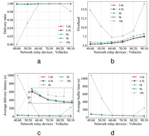
Fig. 7. (a) Delivery ratio versus device ratio (b) Overhead versus device ratio. (c) Average delivery latency versus device ratio. (d) Average buffer time versus device ratio.
