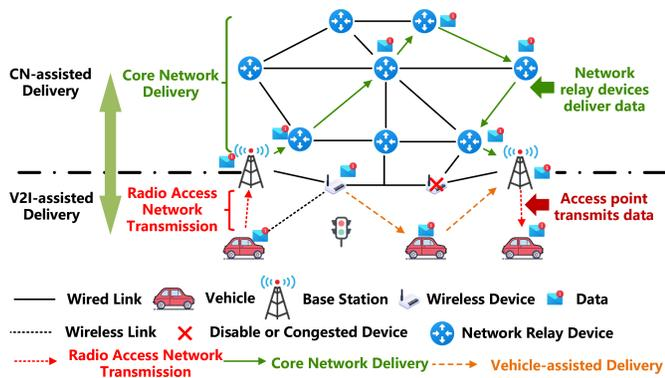
Fig. 1. System Architecture and Data Delivery Model integrated IoVs and CN.
